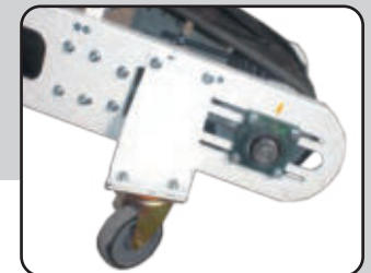
Tail end equipped with two small wheels for maneuvering.
