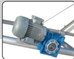
Over 8 meter long Inclined Belt Conveyors Motorized Jack lift is recommend due to load weight.
