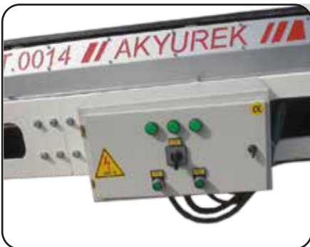
On Board Power Panel
